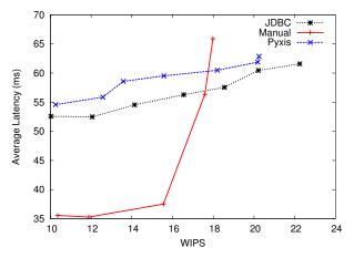
Figure 13: TPC-W latency experiment using 3 cores
